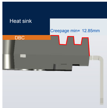
Figure 5. Creepage distance allowed
