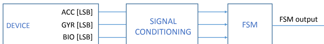
Figure 2. State machine in the ST1VAFE6AX
