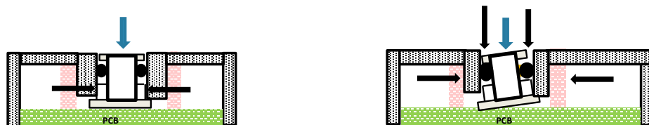
Figure 8. Bad configuration for mechanical stress
