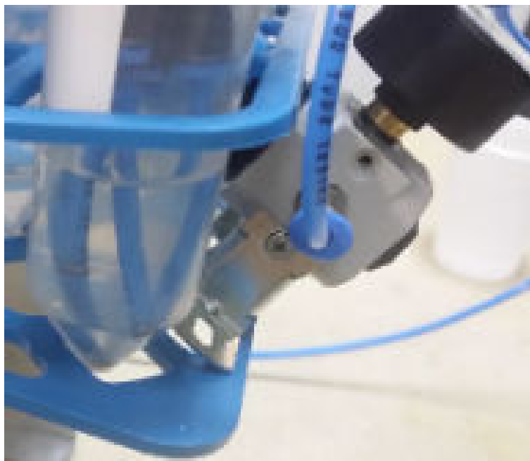
Figure 16. ILPS28QSW immersed in water for air overpressure
