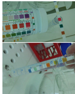
Figure 15. Chlorine, bromine, saltwater and detergent tests
