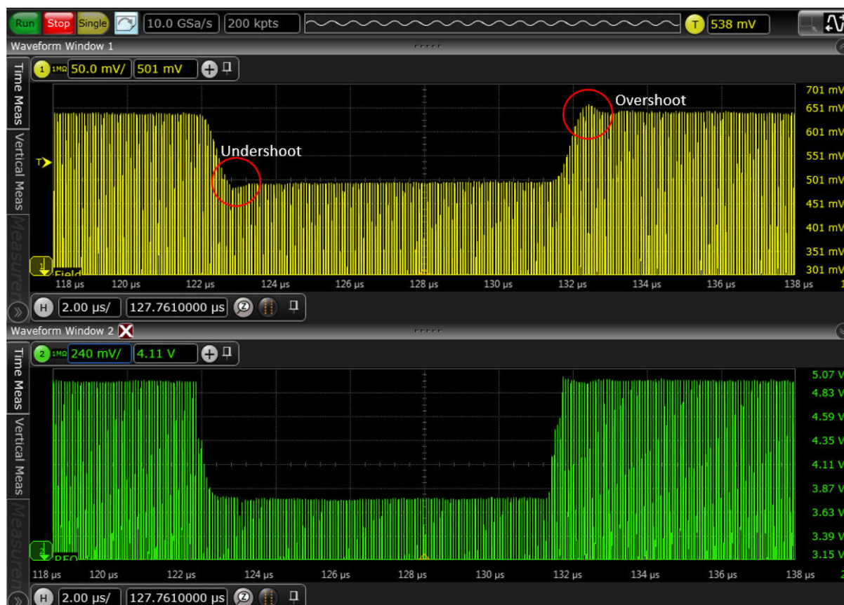
Figure 8. NFC-B modulation with over- and undershoots
