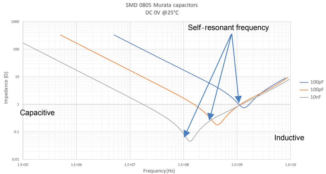
Figure 33. Capacitor impedance vs. frequency
