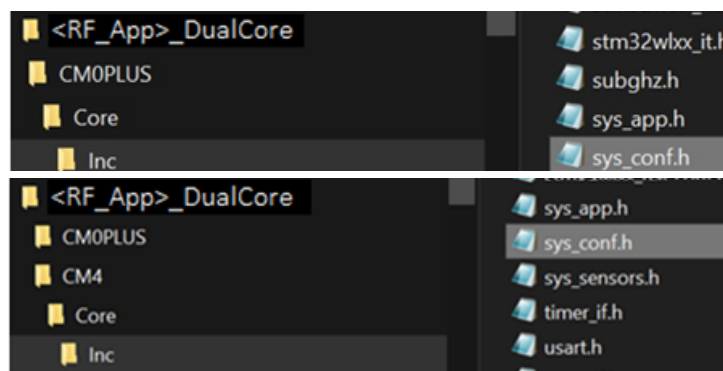
Figure 26. File structure of End_Node dual-core debug configuration
