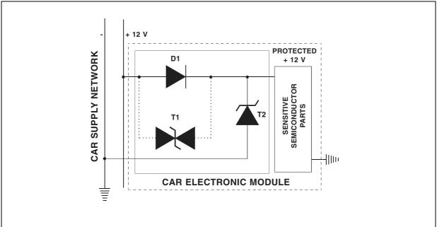
Note that as the voltage across D1 is clamped by T1, the VRRM of the diode is no longer a concern. The clamping voltage is the same as that of T2, given by the yy digits in the part number of the form RBOxxyy. The xx digits indicate the average forward current between pins 1 and 3.
