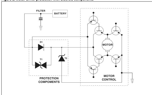
Figure 2. Motor driver protection with discrete components
