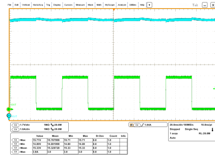
Figure 46. Dynamic load transient zero to full load at V_{OUT} = 15\text{ V} - I_{OUT} = 3\text{ A} ( V_{IN} = 230\text{ V}_{AC} )
