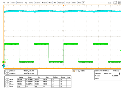
Figure 45. Dynamic load transient zero to full load at V_{OUT} = 15\text{ V} - I_{OUT} = 3\text{ A} ( V_{IN} = 115\text{ V}_{AC} )
