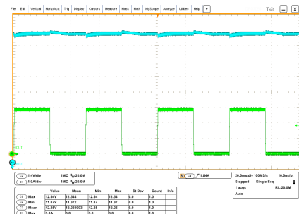
Figure 44. Dynamic load transient zero to full load at V_{OUT} = 12\text{ V} - I_{OUT} = 3\text{ A} ( V_{IN} = 230\text{ V}_{AC} )
