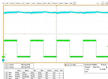
Figure 43. Dynamic load transient zero to full load at V_{OUT} = 12\text{ V} - I_{OUT} = 3\text{ A} ( V_{IN} = 115\text{ V}_{AC} )
