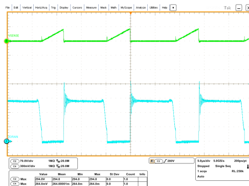
Figure 21. Flyback primary side waveforms at V OUT = 9 V - I OUT = 3 A (V IN = 90 V AC )
