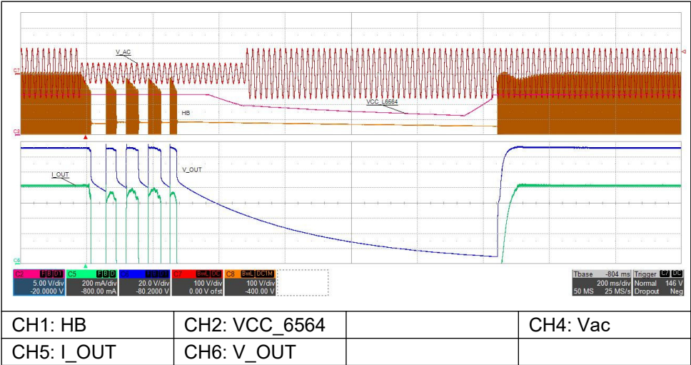
Figure 44. 230 Vac / 50 Hz - full load 10 cycles (200 ms) 40% mains dip (92 Vac)
