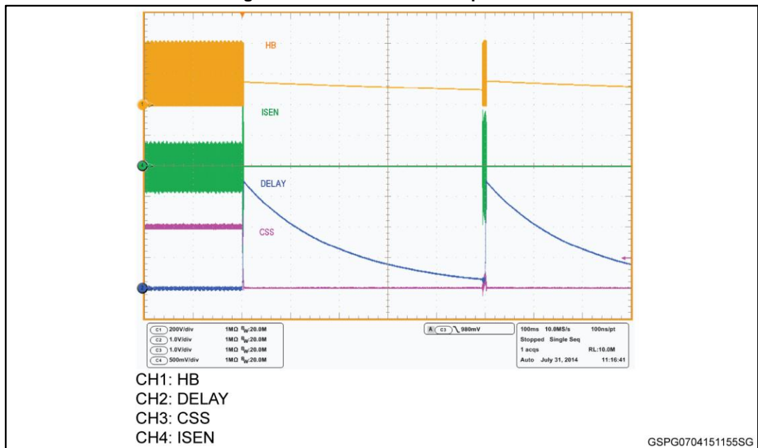
Figure 30: Short-circuit - hiccup mode
