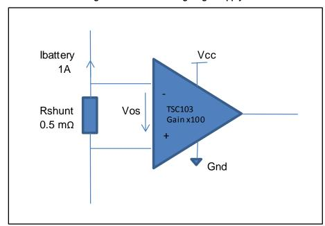
Figure 3: Current sensing single supply
