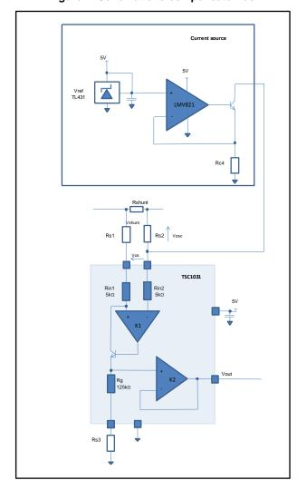
Figure 4: Schematic to compensate Vos
