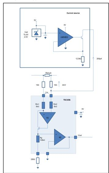
Figure 5: Suggested schematic to compensate Vos
