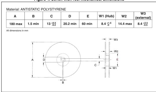
Figure 4. Seven-inch reel mechanical dimensions
