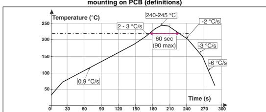
Figure 9. ST ECOPACK® recommended soldering reflow profile for Flip Chip mounting on PCB (definitions)
