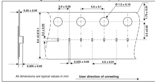
Figure 3. .Tape dimensions for 01005 Flip Chip
