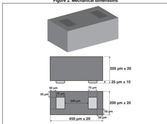
Figure 2. Mechanical dimensions
