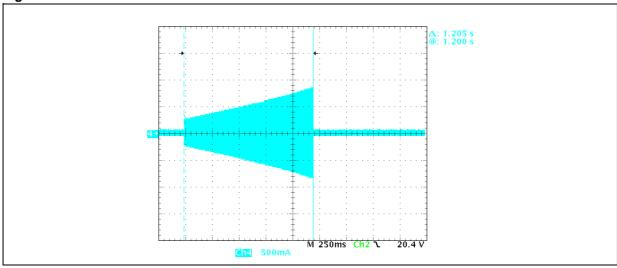
In figure 10 Sec pin voltage and voltage across the preheating capacitor (C12) are shown. Negative Sec pin voltage is clamped at -20V in order to avoid negative over voltage.
