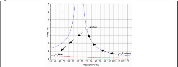
Figure 6 shows the start up phase when pre-heating function is used.
