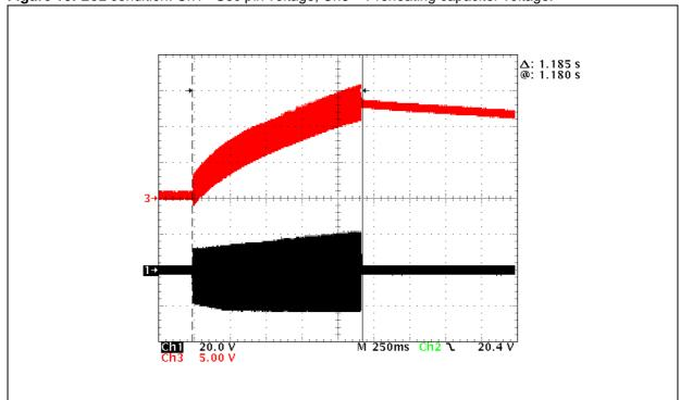
Figure 10: EoL condition. Ch1= Sec pin voltage, Ch3 = Preheating capacitor voltage.
