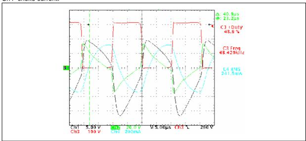
The working frequency is 48 KHz with duty cycle of 49%. Using the proposed input filter the sec pin voltage is higher than 4.5V at the end of Ton time.
