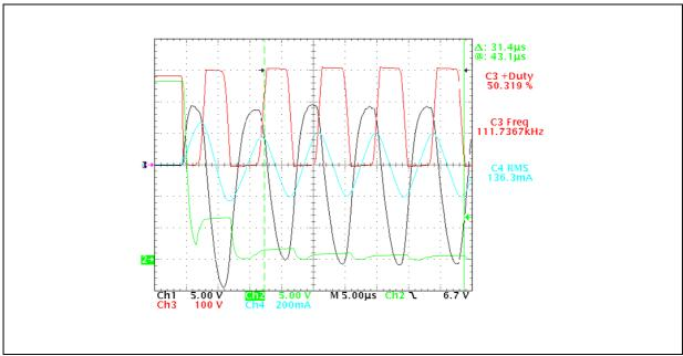
Figure 7 shows the current and the voltage across the cathode during pre-heating. The cathode resistance at the end of the preheating is about 3 times higher than its initial value ensuring the cathodes heating.
