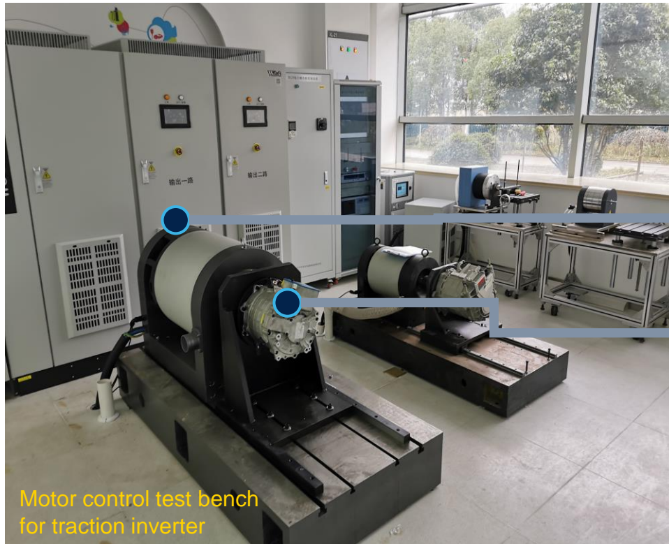
110 kW motor control test bench
